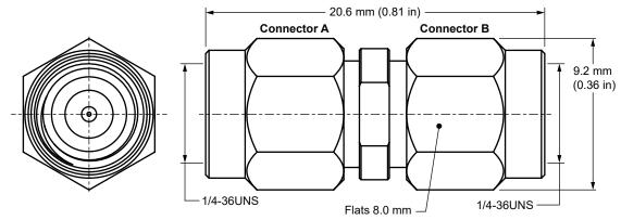
Figure 1. Product Dimensions for the ADP-2.92M-2.92M Adapter
