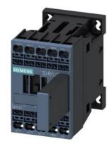
Contactor, AC-3, 7.5 KW / 400 V, 1 NO, 110 V AC, 50 Hz, 120 V, 60 Hz, 3-pole, Size S00 Spring-type terminal RC 3RT2916-1CC00 plugged on
