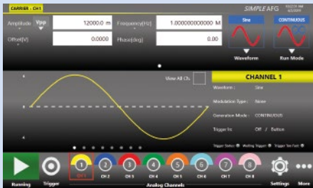
Arbitrary Function Generation (AFG functionality)
