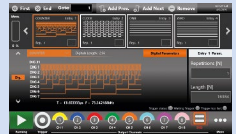
Digital Pattern Generation (DPG functionality)
