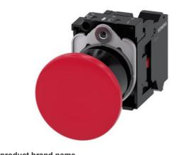
Mushroom pushbutton, 22 mm, round, plastic, red, 40mm, latching, pull-tounlatch mechanism, with holder, 1 NC, spring-type terminal, with laser labeling, inscription or symbol Customer-specific selection with SIRIUS ACT configurator (CIN)
