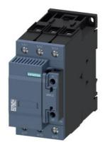
Capacitor contactor, AC-6b 50 kVAr, / 400 V 1 NO + 1 NC, 230 V AC, 50/60 Hz 3-pole, Size S2 screw terminal
