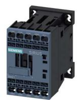
Coupling contactor relay, 2 NO + 2 NC, 24 V DC, 0.7  $\dots$  1.25<sup>\*</sup> US, with integrated suppressor diode, Size S00, Spring-type terminal suitable for PLC outputs
