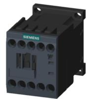
Power contactor, AC-3 12 A, 5.5 kW / 400 V 1 NC, 480 V AC, 60 Hz 3-pole, Size S00 screw terminal
