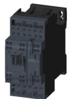
power contactor, AC-3 25 A, 11 kW / 400 V 1 NO + 1 NC, 110 V AC, 50 Hz, 3-pole, Size S0 Spring-type terminal
