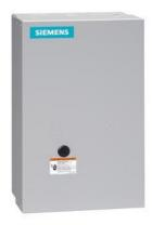
2-speed 3-phase motor starter, Size 0, One winding consequent pole, Constant or variable torque, Solid-state overload relays, Low Spd OLR range 0.75-3.4A, High Spd OLR range 3-12A, Enclosure NEMA type 1, Indoor general purpose use
