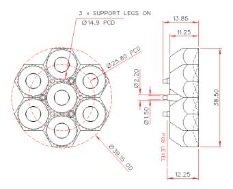
Polymer Optics "Modular LED Optics"<sup>®</sup> design, based on a hexagonal format, allows maximum packing density and assembly flexibility
