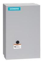
Mechanically held lighting contactor, Contactor amp rating 100A, 0 N.C. / 5 N.O. poles, 110VAC 50HZ/120VAC 60HZ coil, Non-combination type, Enclosure NEMA type 1, Indoor general purpose use
