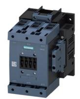
power contactor, AC-3 150 A, 75 kW / 400 V AC (50-60 Hz) / DC operation 23-26 V AC/DC auxiliary contacts 2 NO + 2 NC 3-pole, frame size S6 with box terminal
