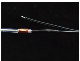
When done correctly the middle wire will be completely protected.
