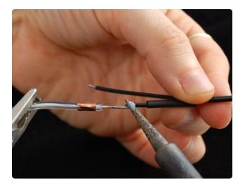
Pull the wire apart so that you can slip the heat shrink on and have 1/4" or more of clearance from the end of the wire, otherwise the soldering iron will prematurely shrink it. Solder the wire to the middle conductor.
