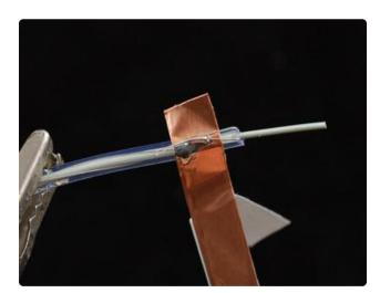
Check that the wires are soldered to the tape.
