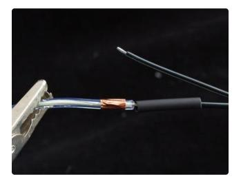
After 15 seconds check that the solder connection has cooled, then slide the 1/8" shrink over the middle joint.
