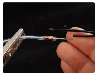
Next get your wire ready, ours come precut and tinned. If not, cut so that one side is about 1/2" longer than the other tin the ends. EL is AC-powered so you dont have to worry about 'polarity'.
