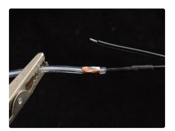
Now we can revisit the corona wires. Using the tip of the soldering iron, heat up the copper tape and melt a little solder on.
