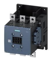
Power contactor, AC-3 265 A, 132 kW / 400 V without coil Auxiliary contacts 2 NO + 2 NC 3-pole, Size S10 Main conductor: Busbar connections Drive: conventional Auxiliary conductor: Screw terminals
