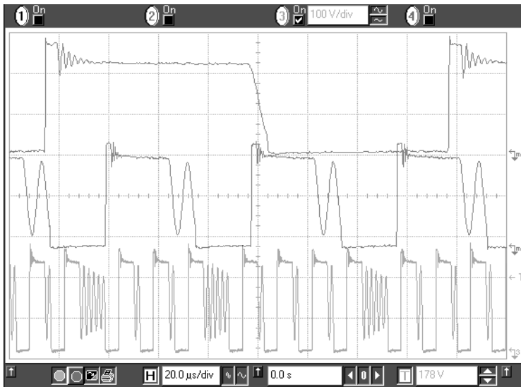
Figure 28. This plot gathers waveforms captured at three different operating points: 1 st Upper Plot: Free run, valley switching operation, P_{out} = 26\text{ W} . 2 nd Middle Plot: Min Toff clamps the switching frequency and selects the second valley. 3 rd Lowest Plot: The skip slices the second valley pattern and will further expand the burst as P_{out} goes low.
