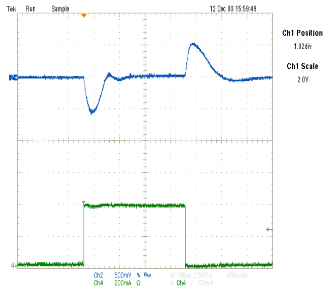
Figure 2–3. TPS65100 Main Boost Converter Load Transient for V_{IN} = 5V and V_{OUT} = 13.5V
