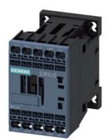
power contactor, AC-3 9 A, 4 kW / 400 V 1 NO, 24 V DC 0.85-1.85\* US, 3-pole, size S00, spring-type terminal not expandable with auxiliary switch
