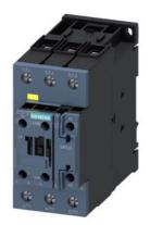
contactor, AC-3, 51 A/400 V/60  $^{\circ}$ C S2, 3-pole, 175-280 V AC/DC, F-PLC-IN, with varistor, 1 NC, screw terminal
