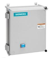
Non-reversing motor starter, Size 1, Three phase full voltage, Solid-state overload relay, OLR amp range 5.5-22A, 240V 50Hz / 277V 60Hz coil, Non-combination type, Enclosure type 4X fiberglass, Water/dust tight noncorrosive, Standard width enclosure
