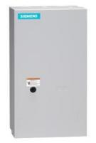
Mechanically held lighting contactor, Contactor amp rating 200A, 0 N.C. / 2 N.O. poles, 208VAC 60HZ coil, Non-combination type, Enclosure NEMA type 1, Indoor general purpose use
