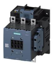
power contactor, AC-3 185 A, 90 kW / 400 V AC (50-60 Hz) / DC operation 21-27 AC/DC, 3 V auxiliary contacts 2 NO + 2 NC 3-pole, frame size S6 busbar connections drive: electronic with PLC interface 24 V DC screw terminal
