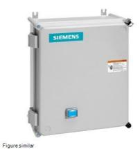
Non-reversing motor starter, Size 2 1/2, Single Phase, 2-Pole, Amb. compensate bimetal OLR, Contactor amp rating 60A, Non-combination type, Enclosure type 4X fiberglass, Water/dust tight noncorrosive
