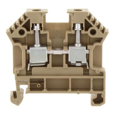
Feed-through terminal, Screw connection, Mounting type: Mounting rail TS 35/7.5, Rated cross-section: 4 mm², Width: 6 mm, Colour: Beige
