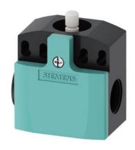
position switch plastic 50 mm increased corrosion protection device connection 2x (M20x 1.5) 1 NO/1 NC integrated (not replaceable) quick-action contacts, rounded plunger, functional at -40  $^{\circ}\text{C}$  shock and vibration test according to EN 61373, category 1B
