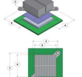
1) Dimension A is the length of the heat sink in the direction of the flow.
