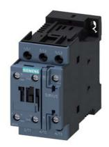
Power contactor, AC-3 38 A, 18.5 kW / 400 V 1 NO + 1 NC, 110 V DC 3-pole, size S0 screw terminals
