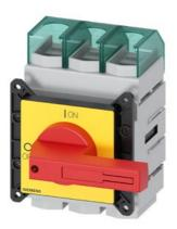
SENTRON, Molded case switch 3LD5 UL, Emergency switching-off, 3-pole, certified according to UL489 UL60947-4-1 and IEC60947-3, UL: 150A, SCCR 50kA at 480VAC, Operating power at 480VAC 3-phase: 100hp, IEC: 160A, Operating power at AC-23A at 400V: 75kW, front-mounted, rotary operating mechanism, red/yellow, 4-hole mounting of the handle, incl. terminal covers for the infeed side
