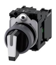
Selector switch, illuminable, 22 mm, round, plastic with metal front ring, white, selector switch, short, 3 switch positions I-O-II, latching, actuating angle 2x45°, 10:30h/12h/13:30h, with holder, 1 NO, 1 NO, screw terminal, with laser labeling, inscription or symbol Customer-specific selection with SIRIUS ACT configurator (CIN)
