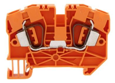
Feed-through terminal, Tension-spring connection, Mounting type: Mounting rail TS 35/7.5, Rated cross-section: 6 mm<sup>2</sup>, Width: 8.1 mm, Colour: Orange
