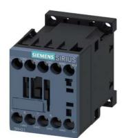
Coupling contactor relay, 4 NO, 24 V DC, 0.7 ... 1.25\* US, with integrated suppressor diode, Size S00, screw terminal suitable for PLC outputs
