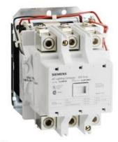
Mechanically held lighting contactor, Contactor amp rating 200A, 0 N.C. / 3 N.O. poles, 220VAC 50HZ/240VAC 60HZ coil, Non-combination type, Enclosure NEMA type (open), No enclosure
