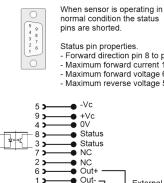
Status pin properties. - Forward direction pin 8 to pin 3 Maximum forward current 10mA - Maximum forward voltage 60V - Maximum reverse voltage 5V
