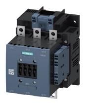
power contactor, AC-3 150 A, 75 kW / 400 V AC (50-60 Hz) / DC operation 23-26 V AC/DC auxiliary contacts 2 NO + 2 NC 3-pole, frame size S6 busbar connections drive: conventional spring-loaded terminal
