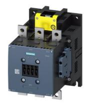
Power contactor, AC-3 300 A, 160 kW / 400 V Coil AC 50/60 Hz and DC 96-127 V x (0.8-1.1) F-PLC input 24 V DC 3-pole size S10 Auxiliary contacts 2 NO + 2 NC Main circuit: Busbar Control and auxiliary circuit: screw terminal
