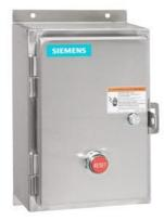
Non-reversing motor starter, Size 1 3/4, Three phase full voltage, Solidstate overload relay, OLR amp range 10-40A, 110V 50Hz / 120V 60Hz coil, Non-combination type, Encl. type 4X 316 S. Steel, Water/dust tight noncorrosive, Standard width enclosure
