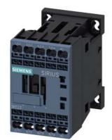
Contactor, AC-1, 22 A/400 V/40  $^\circ\text{C},$  S00, 4-pole, 208 V AC, 50/60 Hz, Spring-type terminal
