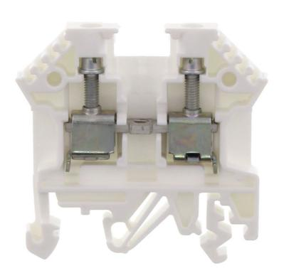
Feed-through terminal, Screw connection, Mounting type:Mounting rail TS 35/7.5 and TS 32, Rated cross-section: 4 mm², Width: 6 mm, Colour: White
