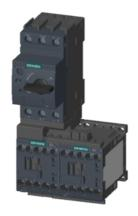
Load feeder fuseless, Reversing duty 400 V AC, Size S00 10.0...16.0 A 230 V AC screw terminal for installation on standard mounting rail Type of coordination 1, lq = 150 kA 1 NC (contactor)
