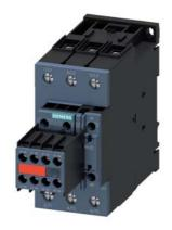
power contactor, AC-3 51 A, 22 kW / 400 V 2 NO + 2 NC, 230 V AC, 50 / 60 Hz, with inserted varistor, 3-pole, size S2, screw terminal captive auxiliary switch
