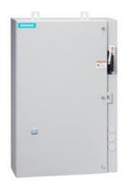
Non-reversing motor starter, Size 2 1/2, Three phase full voltage, Solidstate overload relay, OLR amp range 25-100A, 110V 50Hz / 120V 60Hz coil, Combination type, 100A circuit breaker, Enclosure NEMA type 4/12, Water/dust tight for outdoors, Standard width enclosure
