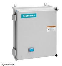
Non-reversing motor starter, Size 2, Three phase full voltage, Solid-state overload relay, OLR amp range 13-52A, Non-combination type, Enclosure type 4X fiberglass, Water/dust tight noncorrosive, Standard width enclosure
