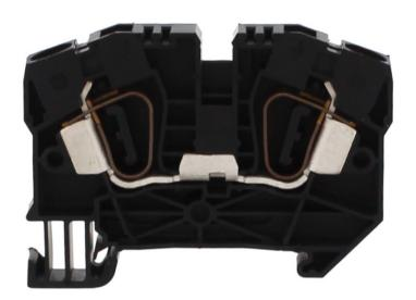
Feed-through terminal, Tension-spring connection, Mounting type: Mounting rail TS 35/7.5, Rated cross-section: 6 mm², Width: 8.1 mm, Colour: Black
