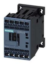
power contactor, AC-3 9 A, 4 kW / 400 V 1 NO, 24 V DC 0.85-1.85\* US, with diode integrated, 3-pole, size S00, spring-type terminal not expandable with auxiliary switch
