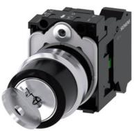
RONIS key-operated switch, 22 mm, round, metal, shiny, lock number SB30, with 2 keys, 2 switch positions O-I, latching, actuating angle 90°, 10:30h/13:30h, key removal O+I, with holder, 1 NO, spring-type terminal, possible special locks: SB31, 421, 455, upper case and lower case, always upper case at beginning of line
