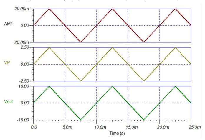
Figure 3. Improved Howland Current Pump Applied as a Peak AC-Current Generator
