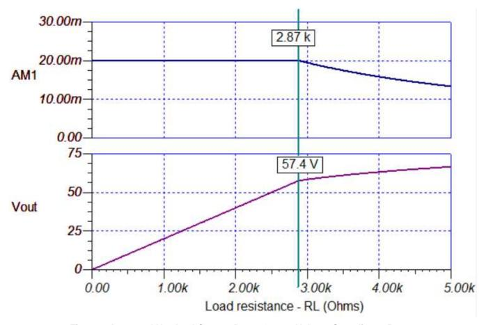
Figure 2. Improved Howland Current Pump Output-Voltage Compliance Range
