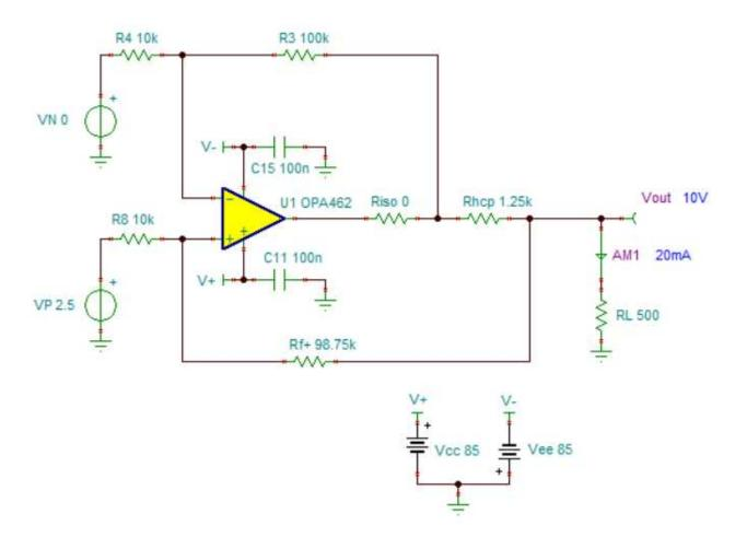
Figure 1. Practical, 20-mA, Improved Howland Current-Pump Circuit
