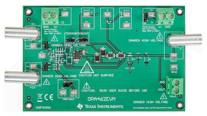
This user's guide describes the characteristics, operation, and use of the evaluation module (EVM) for the OPA462. The EVM is designed to evaluate the performance of the devices in both single and dual-supply configurations. This document also includes the schematic, printed circuit board (PCB) layout, and a bill of materials (BOM). Throughout this document the terms *evaluation board*, *evaluation module*, and *EVM* are synonymous with OPA462EVM.
