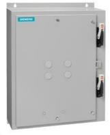
Duplex starter w/ alternator, Size 1, Three phase full voltage, Amb. compensate bimetal OLR, contactor A rating 27A, 110V 50Hz / 120V 60Hz coil, Combination type, Two 10A circuit breakers, Enclosure NEMA type 12, Dust/drip proof for indoors
