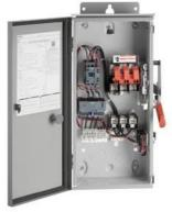
Slim Line Pump Control Panel NEMA size 1 Three phase full voltage Solid-state overload relay OLR amp range 0.75-3.4A 110/120V 50/60Hz Coil 30A fusible disconnect 30A/600V fuse clip 1NC / 1NO auxiliary contacts HOA Sel. Sw. <(>&<)> Start/Stop 3-point power terminal block 3-point control terminal block 3-point ground lug Enclosure NEMA type 3/3R Weather proof outdoor use
